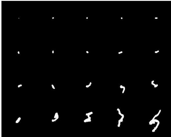
Figure 6. Example showing how the camera-shake pattern changes with exposure duration (from left to right and from top to down, exposure duration increases from 0.01 second to 0.8 second).
