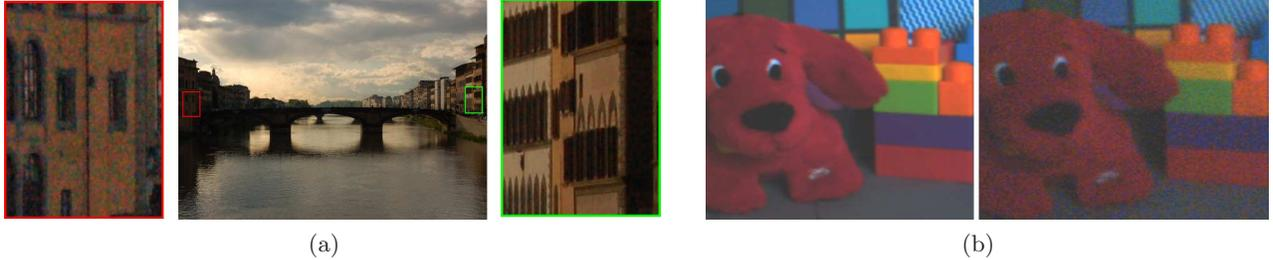
Figure 1. **Image sensor noise from low pixel illumination.** (a) An image acquired with a digital camera under low photopic illumination. Portions of the image from a low-light area (left, red border) and a well-lit area (right, green border) are compared. (b) Simulations of the same scene acquired using a sensor with  $6\ \mu\text{m}$  (left) and  $2\ \mu\text{m}$  (right) pixels.
