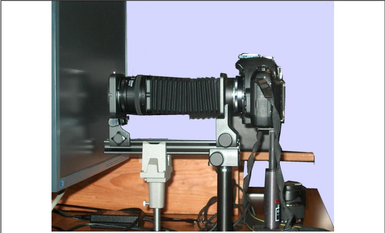
Figure 1. Nikon D100 digital camera with a customized lens and light baffle to measure the spatial distribution of light intensity produced by red, green, blue and white pixels. The lens is a 20 mm focal length objective placed in the reversed direction. In this position, the lens magnifies the pixels by a factor of 10 on the camera sensor.
