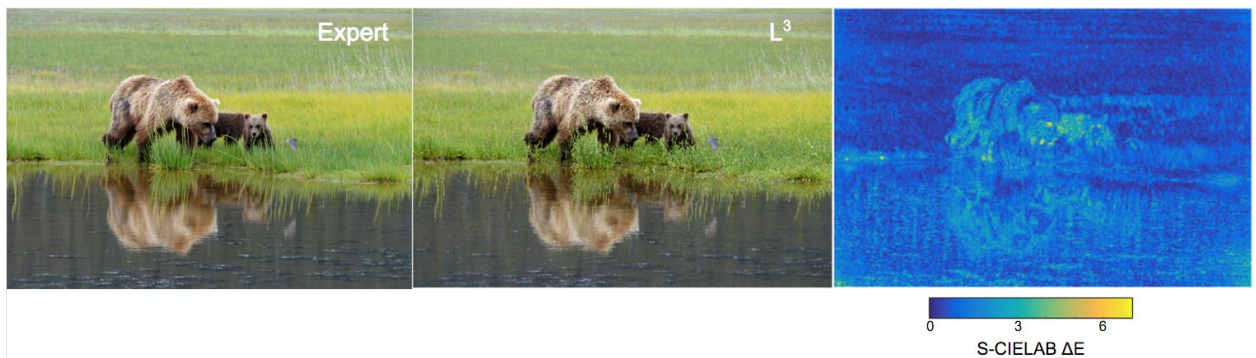
Fig 4. Left: images rendered from the raw sensor data by an expert photography. Middle: Rendering using local linear filters that approximate the rendering by the expert for this image. Right: The S-CIELAB \Delta E_{ab} value for each pixel in the image. The full resolution images for the figures in this paper can be found at [URL]. See text for details.
